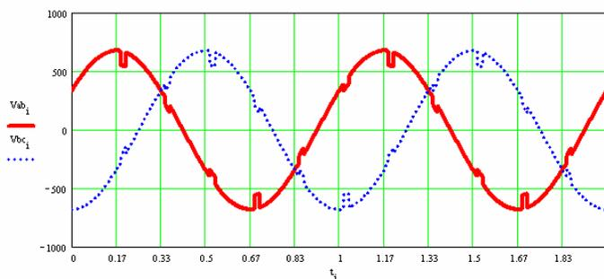
*The typical oscillograph of line to line voltages on the line side of reactors connected to a drive, showing considerably reduced notch depth.*
